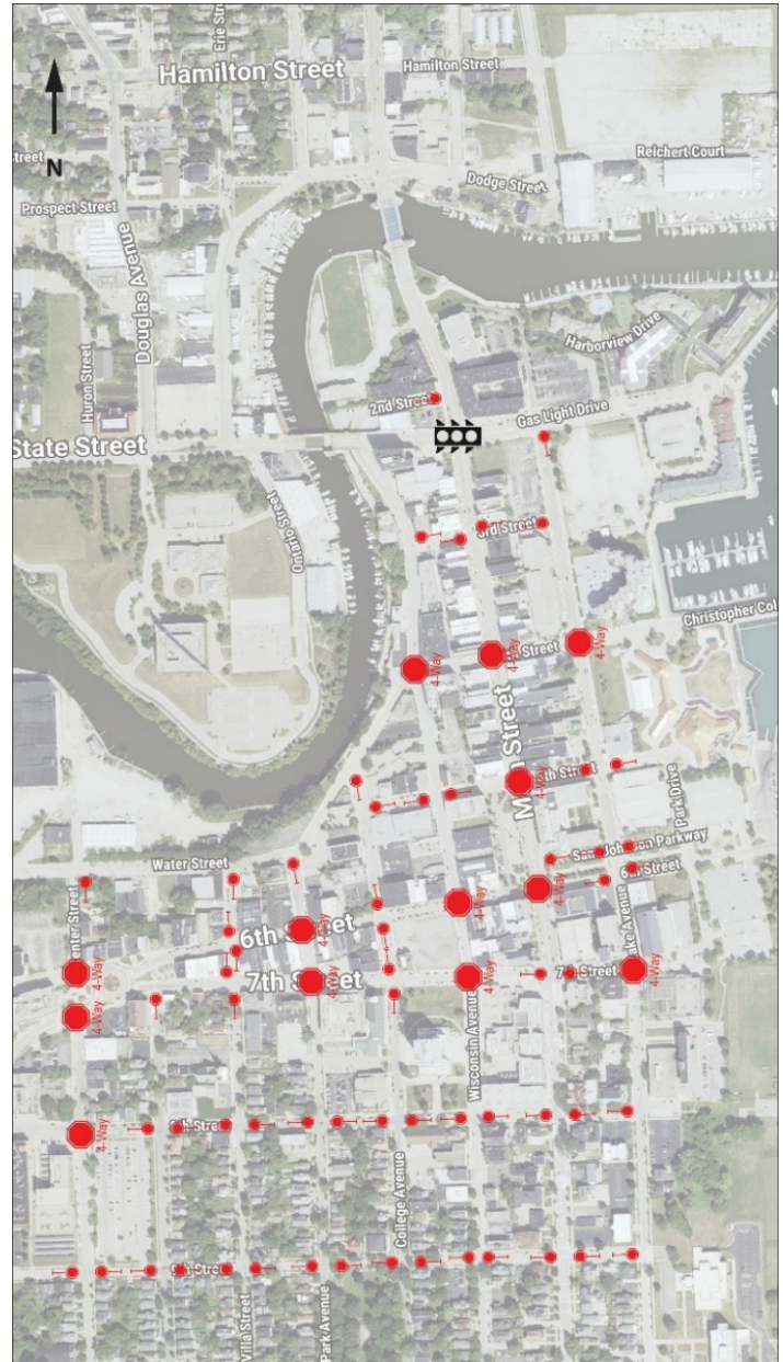
Figure 22: Stop controls after removing one-way operation.
